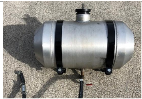
Auxiliary fuel tank, use for extended riding or maintenance, 3.25-gallon spun aluminum - $75.00
